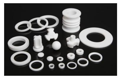
Commonly referred to as Teflon®, PTFE provides true chemical inertness. PTFE is unaffected by most known chemicals, including alkaline solutions, acids and solvents, and also offers extremely low coefficients of friction. Under moderate loads, PTFE can be used in temperatures up to 500°F, and in liquid nitrogen, as low as -325°F.
